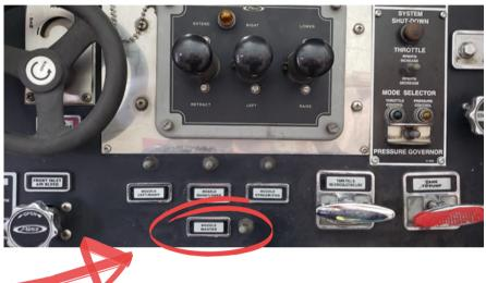
The Nozzle Master switch on the Aerial platform must also be in the up or forward position
