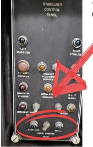
The Aerial Diverter switch must be set to "Stabilizer" to extend the outriggers. When they are set, switch over to "Aerial" to control the ladder
