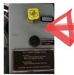
Apply the parking brake and front wheel lock. You need to hold the front wheel lock down for several seconds to get it to engage.
