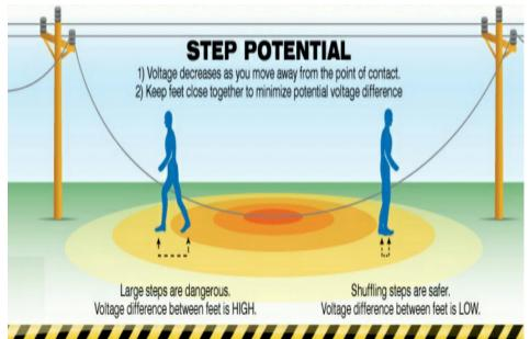
Continue shuffling until you are a safe distance away: **at least 30 feet away** from a downed distribution line (found in neighborhoods) and **at least 100 feet away** from a downed transmission line (found on large towers). These clearance distances are minimums; always use the maximum possible clearance.<sup>2</sup> Never move closer to a downed line; only use this method as a means of escape.
