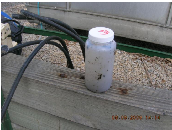
Figure 20 – Sample container from upstream manhole 03-81 US1 (2009)
