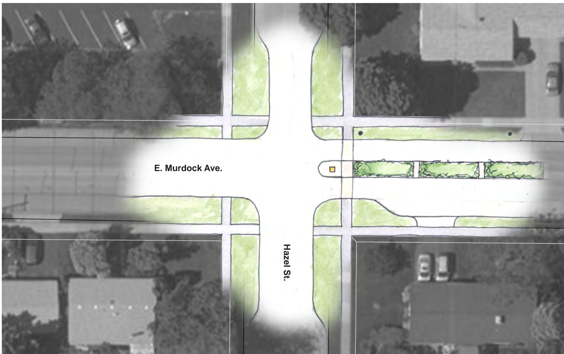
Concept sketch showing a potential median planting, separating traffic as it travels E. Murdock Avenue.
