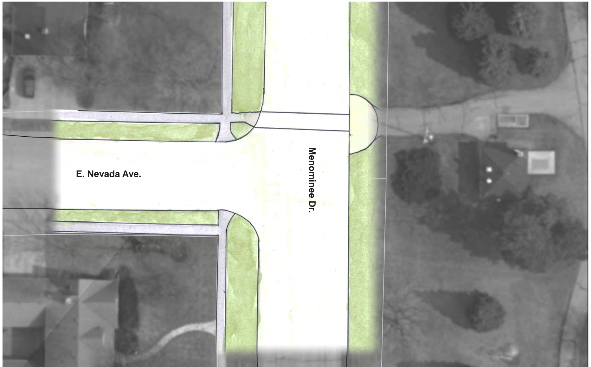
Concept sketch showing a mountable curb into Menominee Park to maintain maintenance vehicle access.
