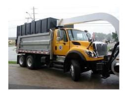
2022-replace #69, a 2011 International, with a tandem-axle plow truck with stainless steel box, prewet, wing, and tailgate spreader. The tailgate spreader is lower maintenance and easier to install than the slide-in spreader it's replacing.
