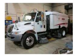
2023-replace #157, a 2013 Elgin Whirlwind street sweeper. A more efficient vacuum sweeper will help the City with clean water initiatives. The pollutants resulting from traffic and road maintenance become attached to pavement dirt particles, which then wash into storm sewers after a rainfall. By controlling the build-up of dirt on our roads, levels of pollutant wash-off can be reduced.
