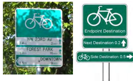
Signs with travel time and distance information to inform cyclists how long a bicycle trip will take
