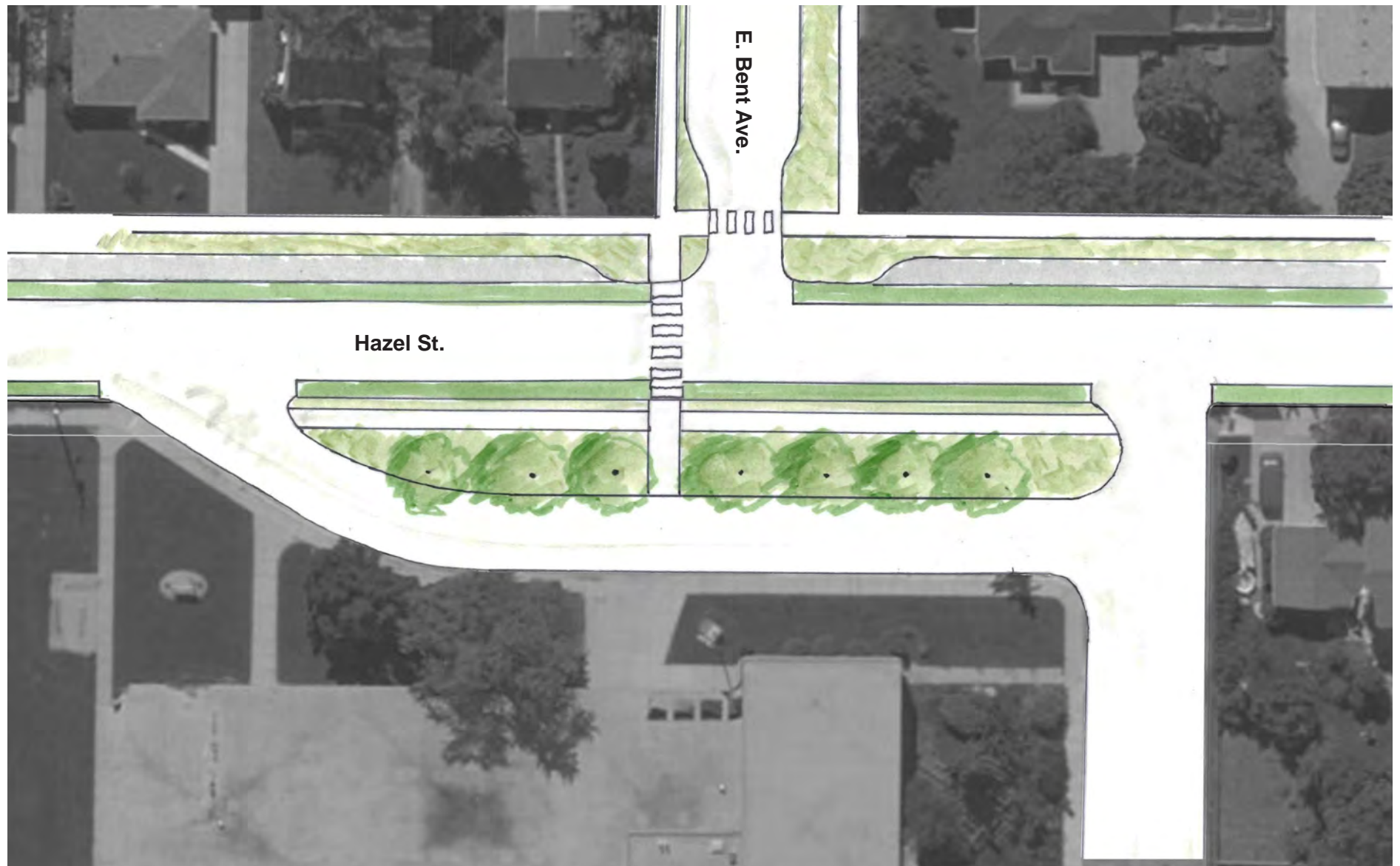
Concept sketch showing potential bike lanes and bumpouts along Hazel Street, directly in front of Emmeline Cook School.
