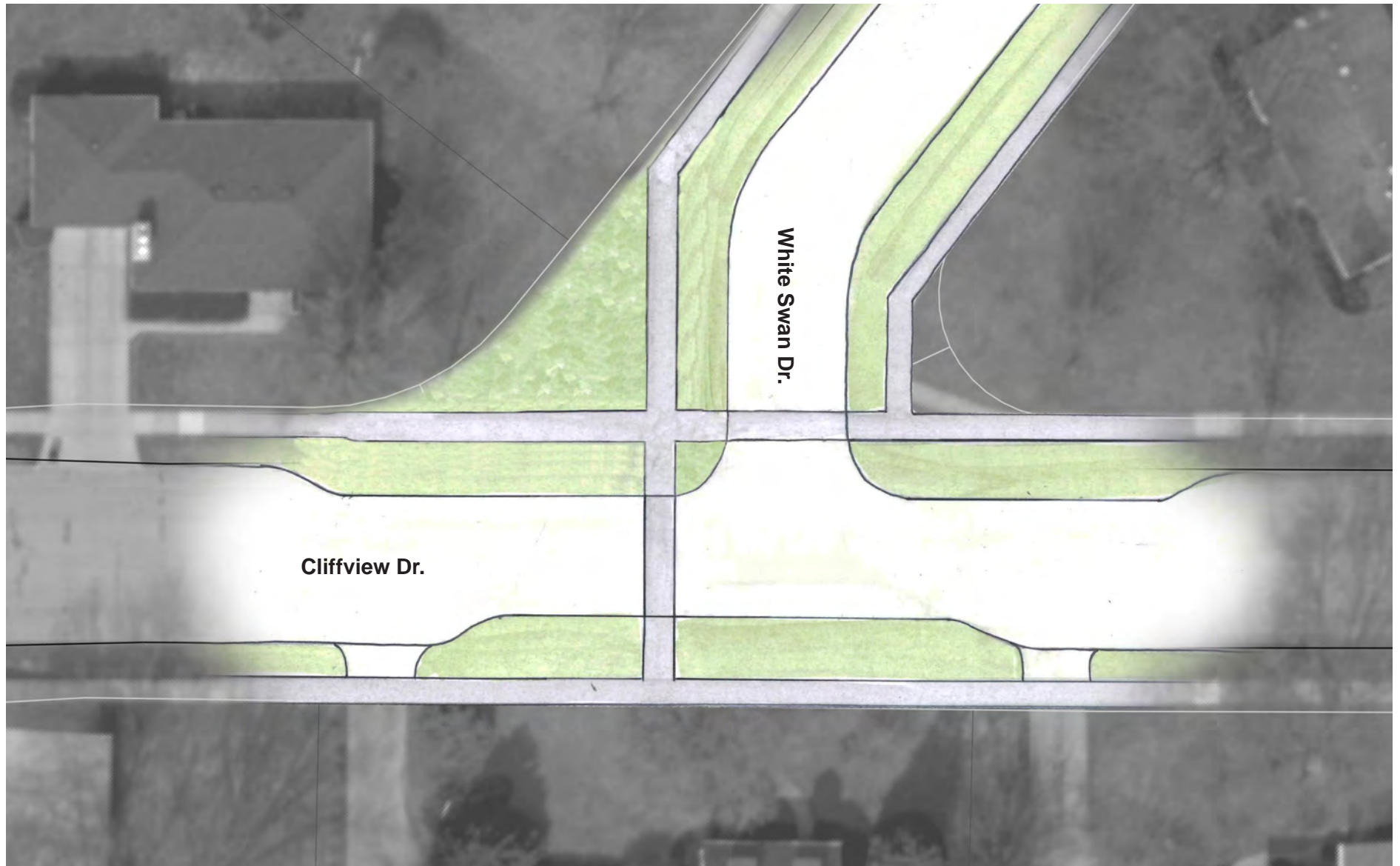
Concept sketch showing how much additional green space is created by re-aligning the White Swan intersection.
