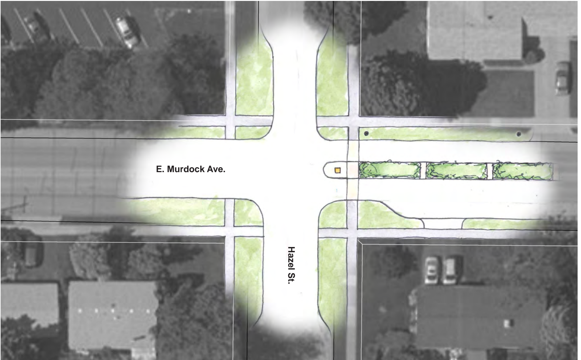
Concept sketch showing a potential median planting, separating traffic as it travels E. Murdock Avenue.
